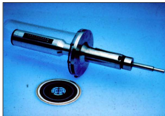
Figure 5-11 Waterproof Rebound Hammer
