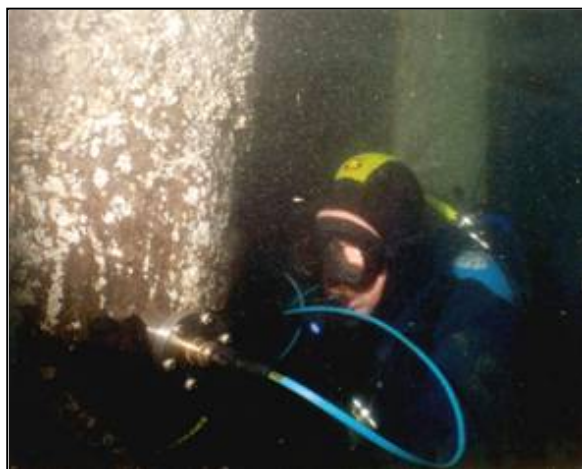
Figure 5-9 Diver Applying the Transducers to a Pile for the Direct Transmission Method
