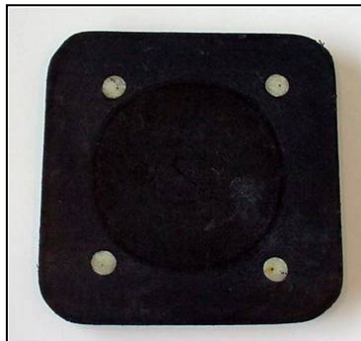
Figure 3-7 Cross Section of Load Bearing Composite Pile
