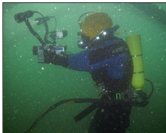
Figure 4-15 Video Camera in Housing with Monitor
