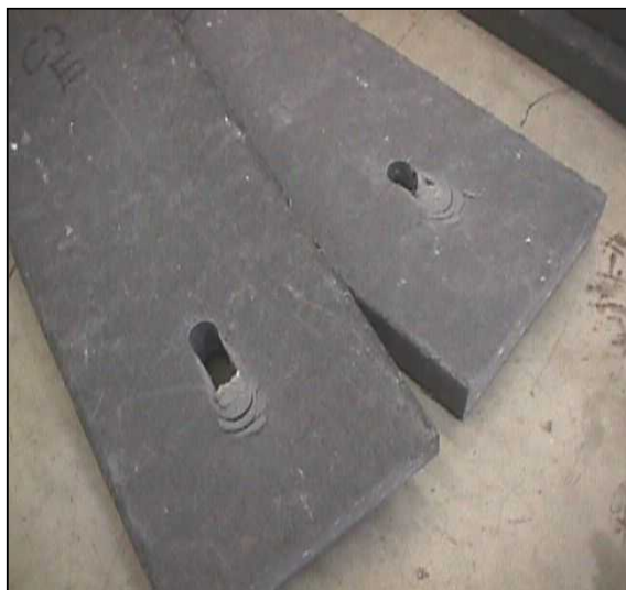
Figure 3-38 Yielding Around Hole of Composite Member
